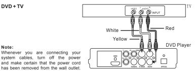
has been removed from the wall outlet 1. Connect the audio cables to the AUDIO OUT L and R jacks on the back of your DVD player and to the corresponding AUDIO INPUT jacks on your TV.
